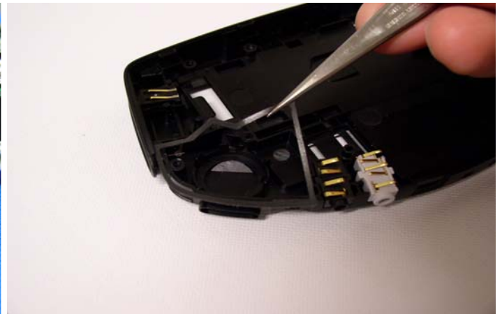
Replace damaged or loose silicon gasket with a spare part gasket. Fix the gasket carefully with tweezers in chassis.
