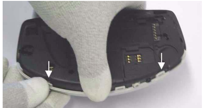
The A-Cover is attached with snaps. Open both snaps before removing A-cover.
