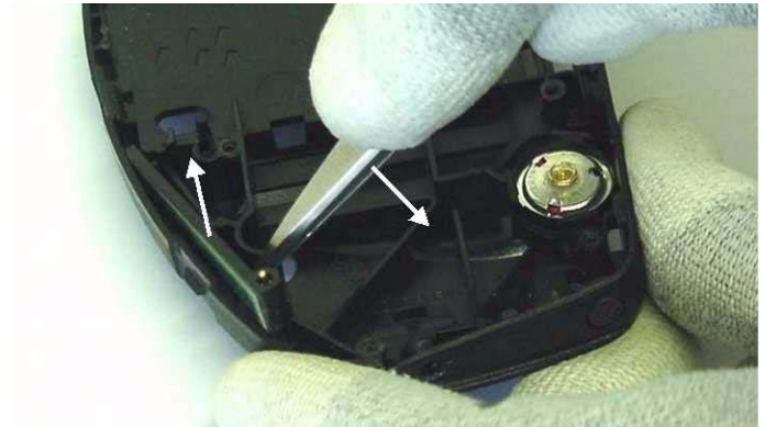
Remove Antenna from Chassis with tweezers.
