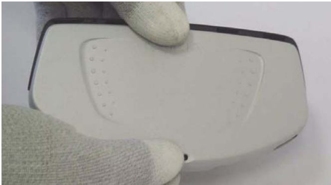
Press the Release Button before removing B-Cover.
