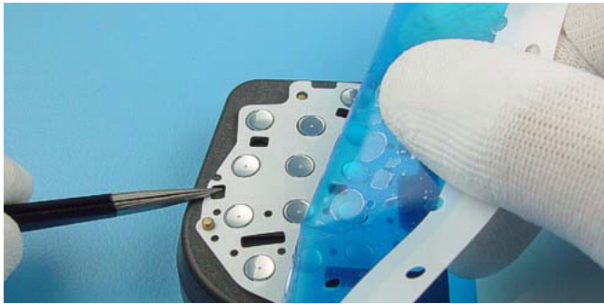
Remove the protection film. Tweezers can be used for retaining the Dome Sheet.
