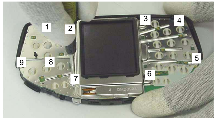
Unscrew the Torx PLUS size 6 screws, using the order shown. For assembly, take reverse order and torque of 26Ncm. Press down the PWB with fingers.
