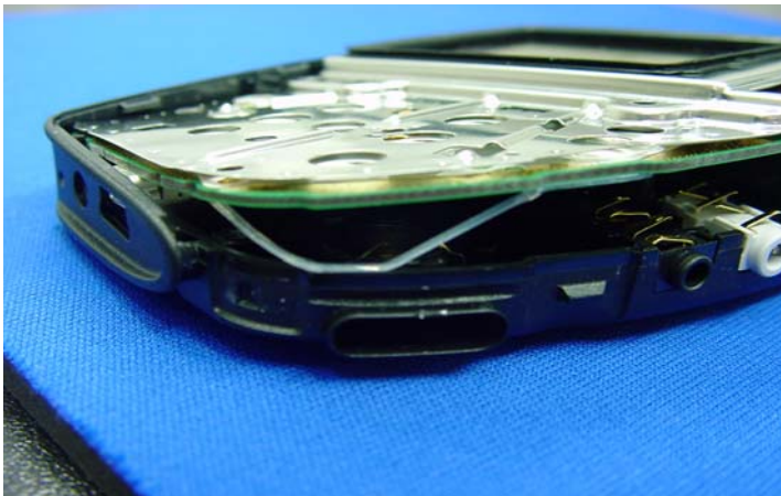
Note! The silicon gasket may stick in the PWB. Damaged and loose silicon gasket must be replaced with a spare part gasket.
