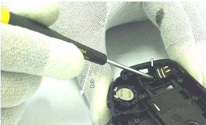
Remove DC Connector from Chassis with Torx. Put Torx under the DC Connector (1) and bend (2).
