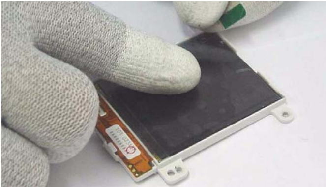
Always protect LCD with protection foil to avoid dust and scratches.
