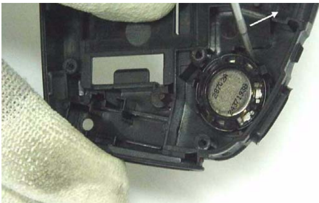
Remove HF Speaker from Chassis with screwdriver. Put screwdriver between Chassis and HF Speaker then bend screwdriver. Take care not to damage the snaps by bending them too much.
