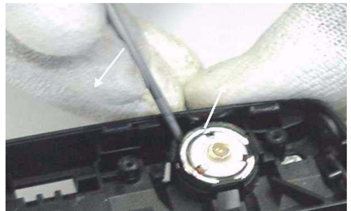
Remove Earpiece with screwdriver from Chassis by bending the snaps carefully.
